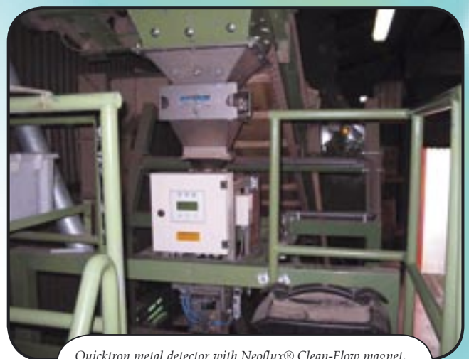
Quicktron metal detector with Neoflux® Clean-Flow magnet. This can be cleaned manually and acts as a pre-separator.
