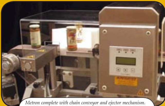
Metron complete with chain conveyor and ejector mechanism. In case of detection a cylinder pushes the product from the belt.
