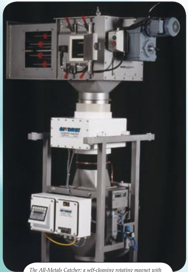
The All-Metals Catcher: a self-cleaning rotating magnet with a Quicktron metal detector. This system is used under a silo just before the loading of the truck. Product: milk powder.
