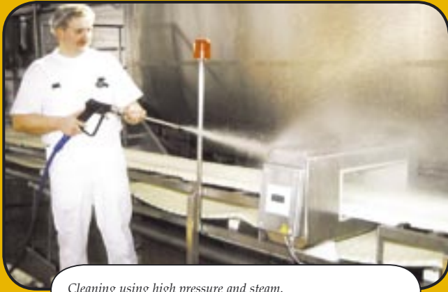
Cleaning using high pressure and steam.
